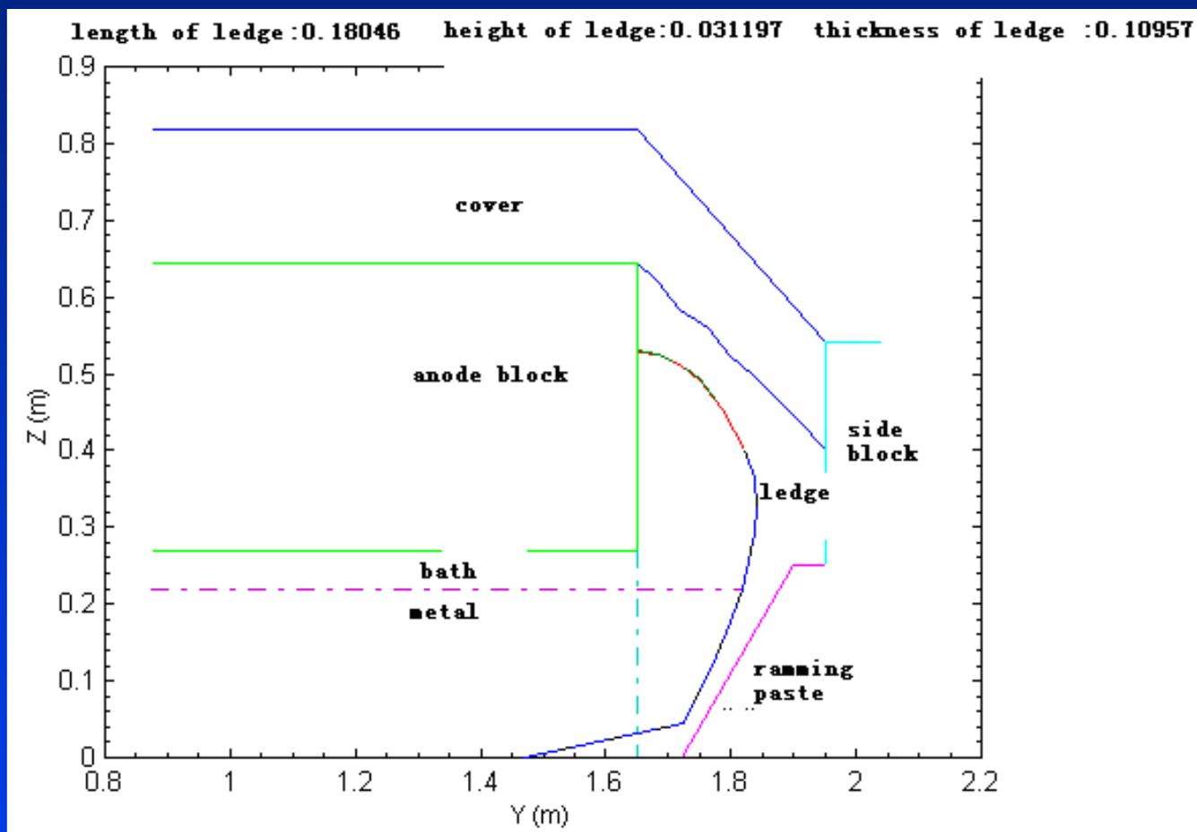
Conventional lining structure, profile of pot side ledge
