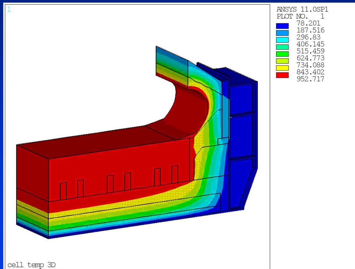
Conventional lining structure, pot end temperature
