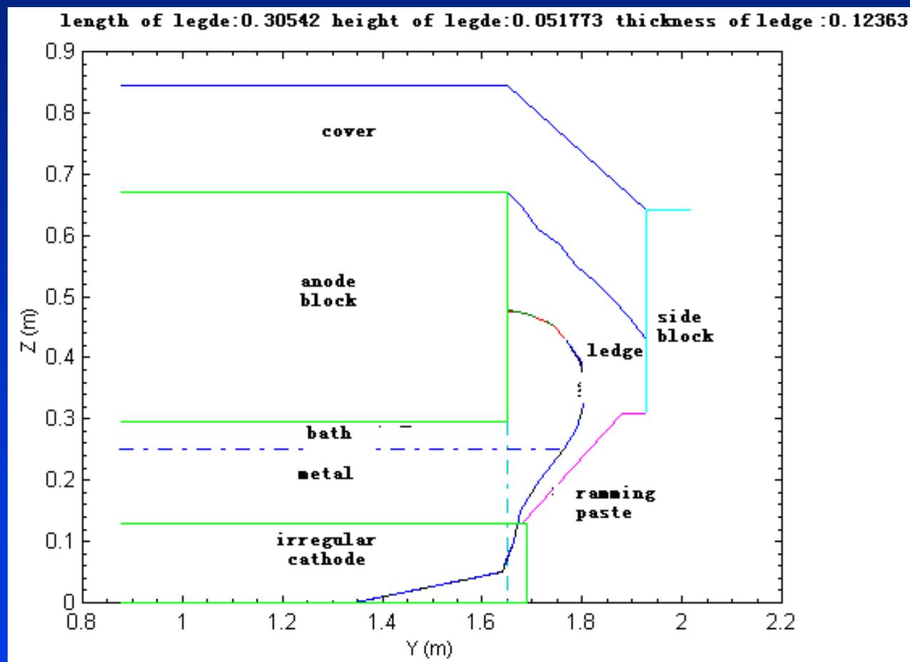
New thermal insulation lining structure, profile of pot side ledge
