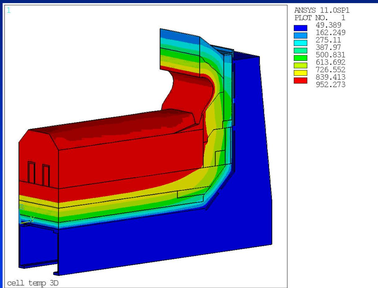
New thermal insulation lining structure, pot side temperature
