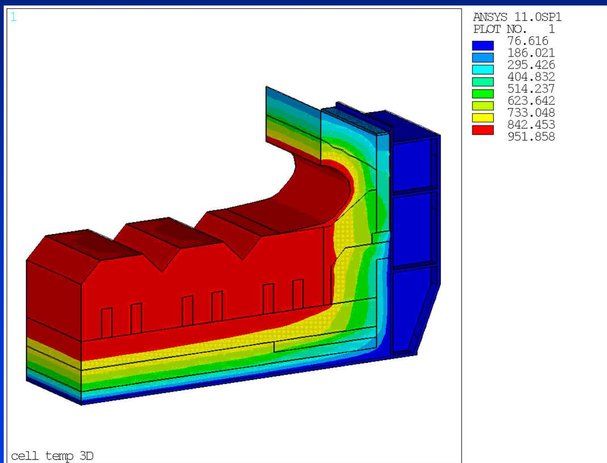
New thermal insulation lining structure, pot end temperature
