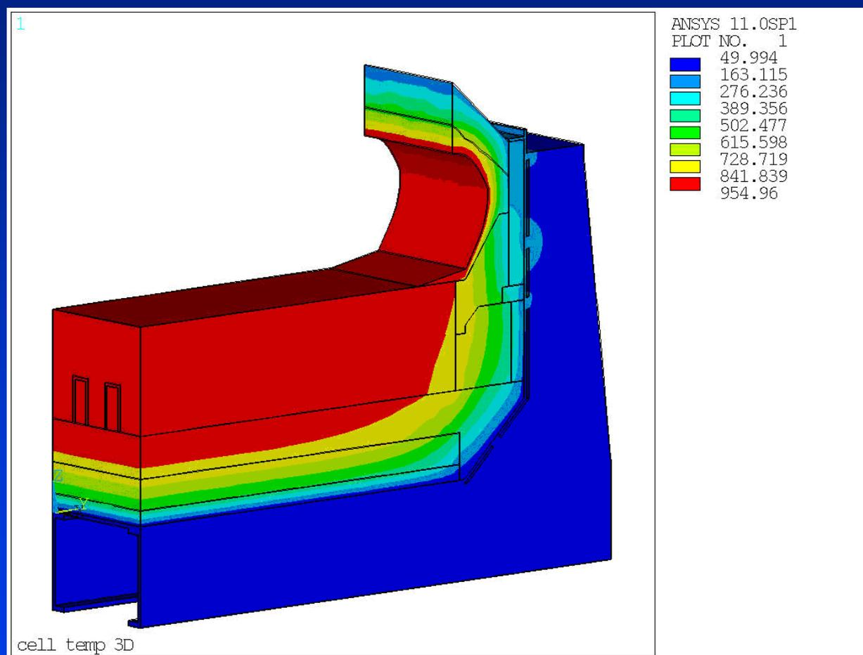
Conventional lining structure, pot side temperature
